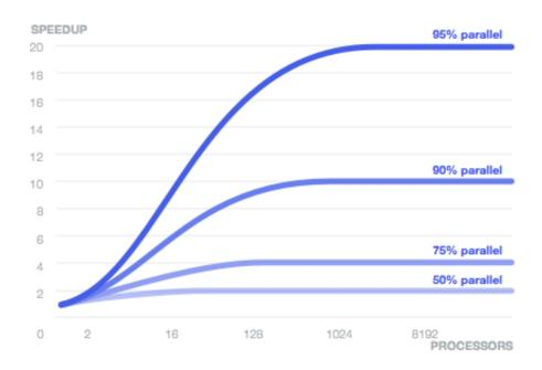
The speedup of a program using multiple processors in parallel computing is limited by the sequential fraction of the program. For example, if 95% of the program can be parallelized, the theoretical maximum speedup using parallel
